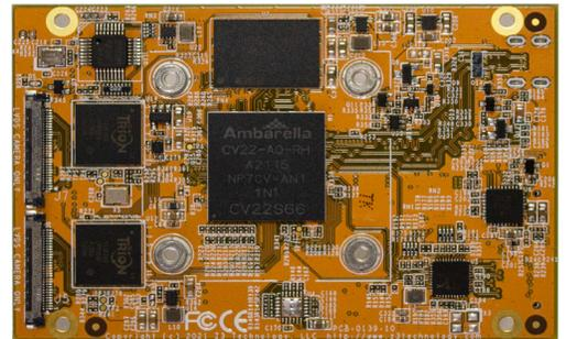
The FV2K-13A designed for dual camera inspection, surveillance, industrial and UAV applications. The flexibility of the system allows for a visible camera and an infrared or night vision camera. The hardware consists of a 2-board set: Encoder and Connector PCB. The system is capable of encoding multiple channels of H.265 or H.264 video in HD resolutions. The Input board features flexible digital and analog input ports. The encoder can be configured to stream over IP and simultaneously record.
